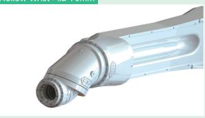
Hollow wrist arms can be applied with internal hoses, reducing the risk of contaminants in the paint finish. The inner diameter of the hollow wrist is 70mm.
