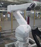
The control system for painting robots can control inner pressure of a manipulator by air-purge control to meet the safety regulation of explosive-proof certification also monitor the status.
